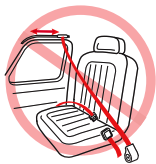
Lap Belt with Motorized Shoulder Belt
